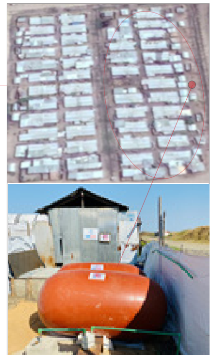
Circled area showing 20 shelters for cooking in block T2, of sector 2 in Malakal PoC. Each shelter has 4 households therefore, a total of 80 households use biogas for cooking on a 20-day rotational cooking plan.
