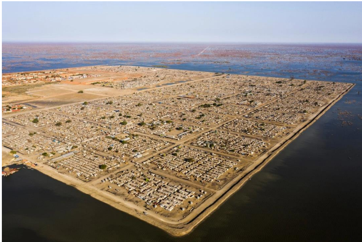
Figure 4.1: Dikes protect the main IDP (internally displaced persons) camp in Bentiu
